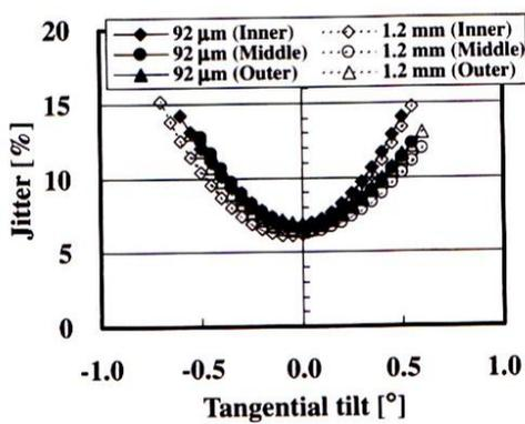
Fig.7 Tangential tilt margin curves of 92um SVOD and 1.2mm product disk. These are overlapped. Thus, thin disk can be used as a standard disk.
