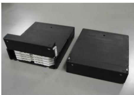
Fig.12 Cartridge of SVOD with 48 disks.
