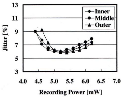
Fig.11 Recording power margin of thin BD type SVOD.
