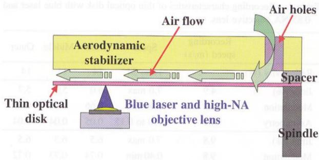
Fig.3 Aerodynamic stabilizer is mounted on the disk.
