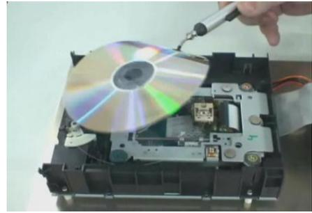
Fig.2 Thin film disk is put on the motor of commercialized standard BD drive.
