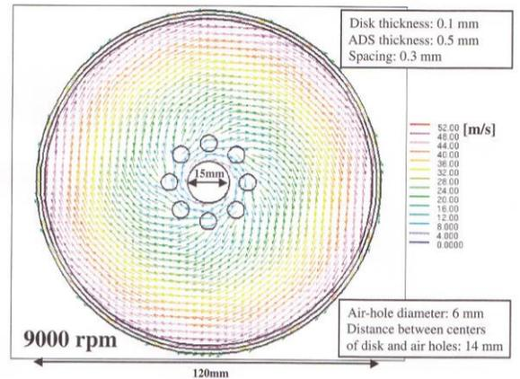
Fig.4 Aerodynamic stabilizer with inner holes.
