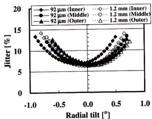
Fig.8 Radial margin curves of thin disk. These are overlapped. This shows that thin disk can be used as a standard disk.
