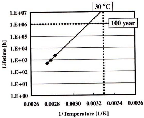
Fig.9 Arrhenius plot of thin disk for durability test.
