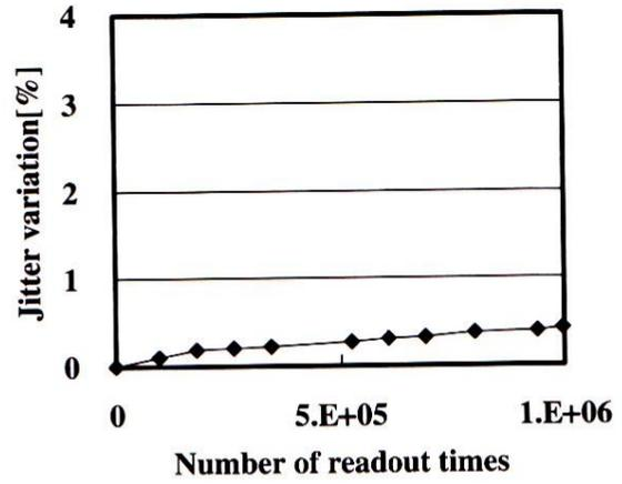
Fig.10 Readout power durability test of thin disk.
