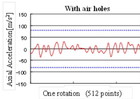
Fig.6 Axial acceleration with inner holes. The experimental result is in the spec.. Air flow keeps flat disk rotation.
