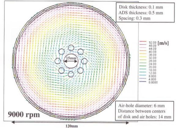
Fig.4 Aerodynamic stabilizer with inner holes.
