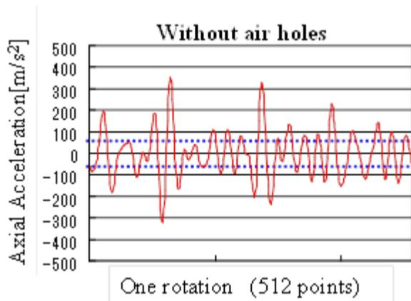
Fig.5 Axial acceleration without inner holes. Dashed line is the specification, and the experimental result is over the spec..
