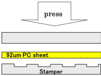
Fig.1 Schematic figure of nano-imprint
