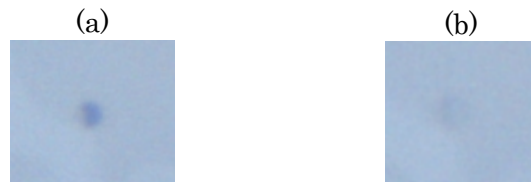
Figure 1 Microscopic photos of the N-doped GeTe thin film; (a) amorphous mark, and (b) erased mark by the crystallization
