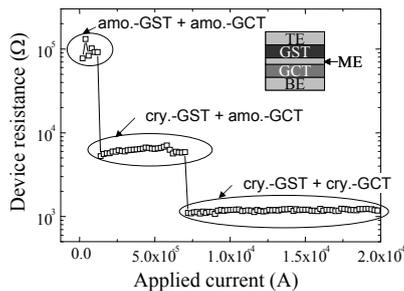
Fig.2. R-I characteristic of memory cell with GST and GCT. Here, three resistance states are confirmed. TE, ME and BE indicate top, middle and bottom electrodes.
