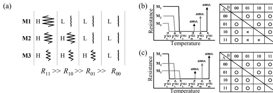
Fig.1. (a) Multi-level states in a combination of M1, M2 and M3 materials, where H and L mean high and low resistance, respectively. (b)(c) Combination of multiple phase change materials with different melting point and crystallization temperature.  $T_x$  and  $T_m$  indicate crystallization and melting temperatures. ×:direct transition (A→B) is impossible. ○:direct transition (A→B) is possible.
