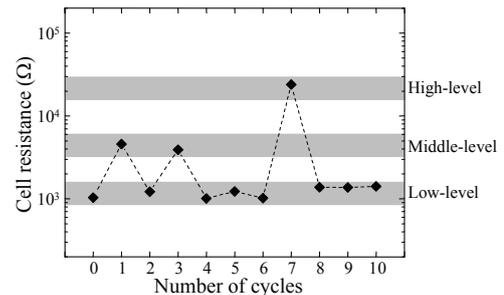
Fig.3. Cyclic characteristic of the multi-layer cell. Three-state transition was confirmed by controlling the applying electrical pulse.
