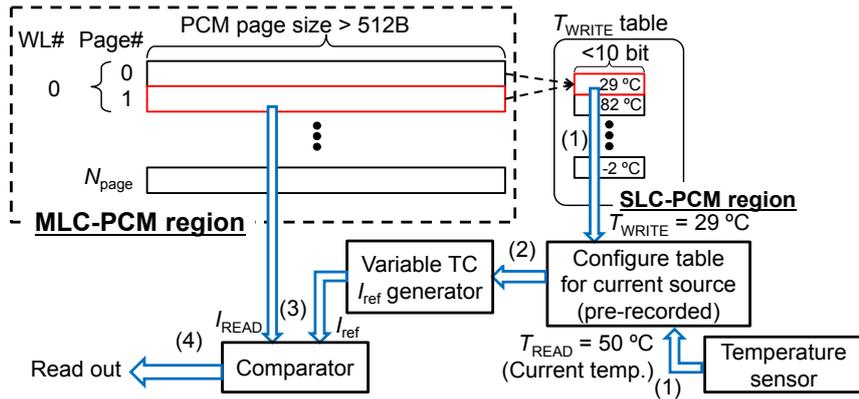
Fig. 3 Block diagram of the proposed read circuit for MLC-PCM.
