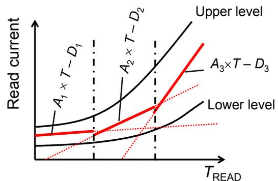
Fig. 2 Concept of the proposed exponential reference current generator.
