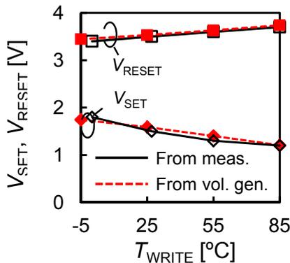
Fig. 1 Measured temperature dependence and fitting result of SET and RESET voltage
