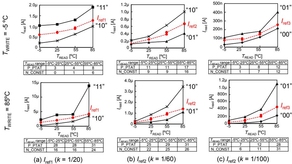
Fig. 4 Demonstration results of read reference current generation for 2 bit-MLC-PCM.
