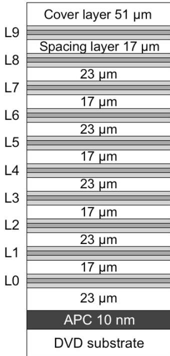
Figure 1 Stacking structure of Disk B. Lx (x=0–9) are the recording layers and each consists of ZnS-SiO<sub>2</sub>/IAO/ZnS-SiO<sub>2</sub>.
