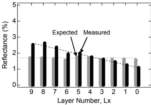
Figure 3 Reflectance of each recording layer (L0–L9) for Disk B (gray: expected, black: measured).
