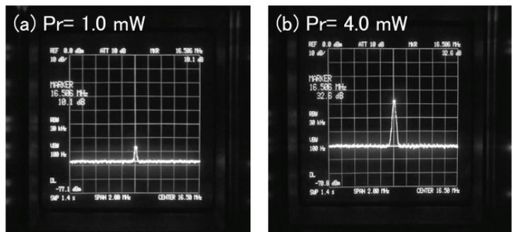
Figure 4 CNR of 113 nm marks for Disk B at L5. Readout laser power (Pr) was 1.0 mW (a) and 4.0 mW (b).
