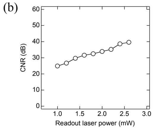
Figure 2 CNR properties of Disk A as a function of mark length (a) and readout laser power for the 112 nm mark (b).
