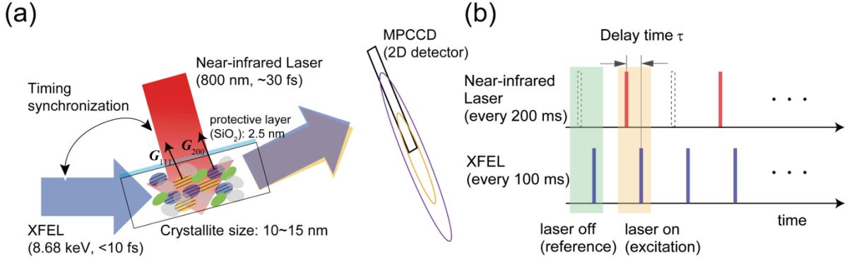
**Figure 2** (a) The optical geometry and (b) procedure of the NIR pump and X-ray probe measurements.
