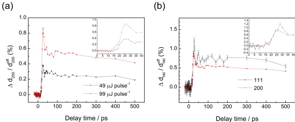
**Figure 4** (a) NIR laser fluence difference of time evolution of expansion calculated from 200 reflections. (b) Directional difference of time evolution of expansion at same NIR laser fluence ( $99 \mu\text{J pulse}^{-1}$ ).
