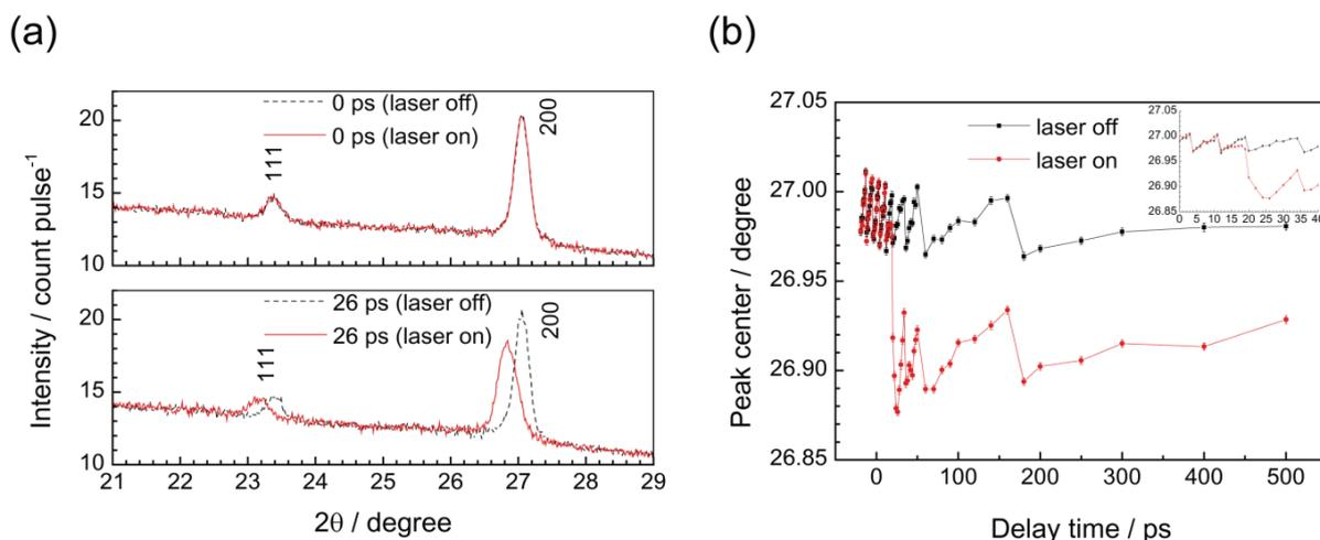
**Figure 3** (a) Typical XRPD profiles of laser off (reference) and on (excited), 500 shot averaged and 1D-converted. (b) Time evolution of peak center position of 200 reflection of laser off and on. Minus delay time means that XFEL arrives earlier than NIR laser. The inset is magnified at earlier stage.
