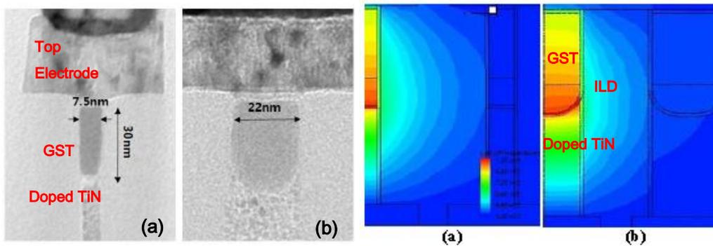
Fig. 3 Cross sectional TEM images of 20nm confined cell and temperature profile of confined cell along BL direction (a) WL direction and (b) BL direction.
