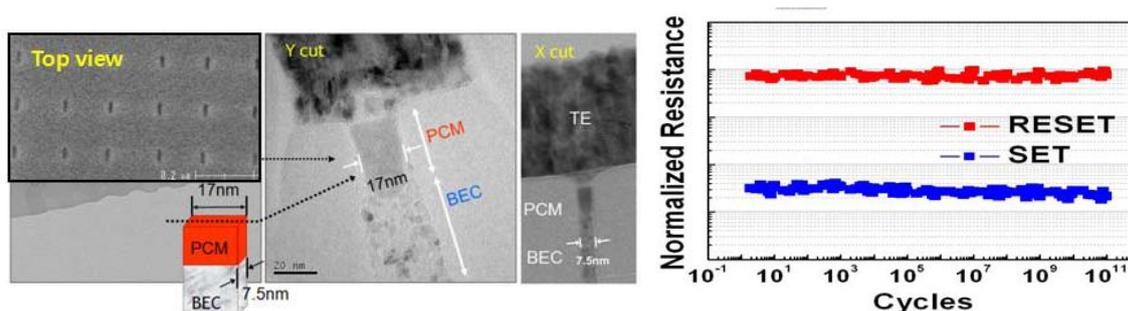
Fig. 6 Confined cell structure was shown. The memory volume was fully isolated in confined cell structure. And its endurance characteristics showed no failure until  $10^{11}$  cycles.
