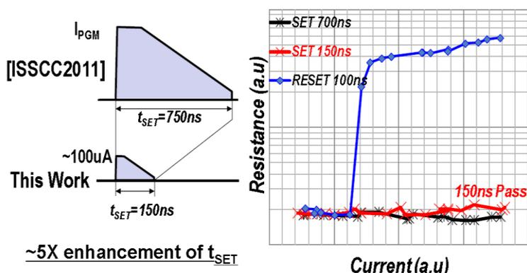
Fig. 5 Resistance-current curve of 20nm confined cell as a function of  $t_{SET}$ .
