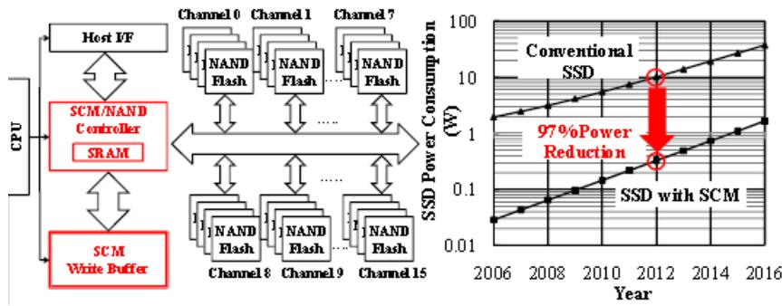
Fig. 2 SCM & NAND flash memory hybrid SSD system [1].
