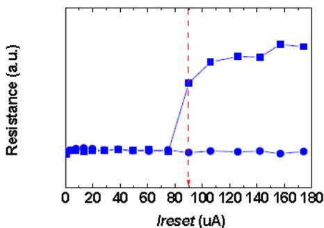
Fig. 4 Resistance-Current curve of 20nm confined cell.
