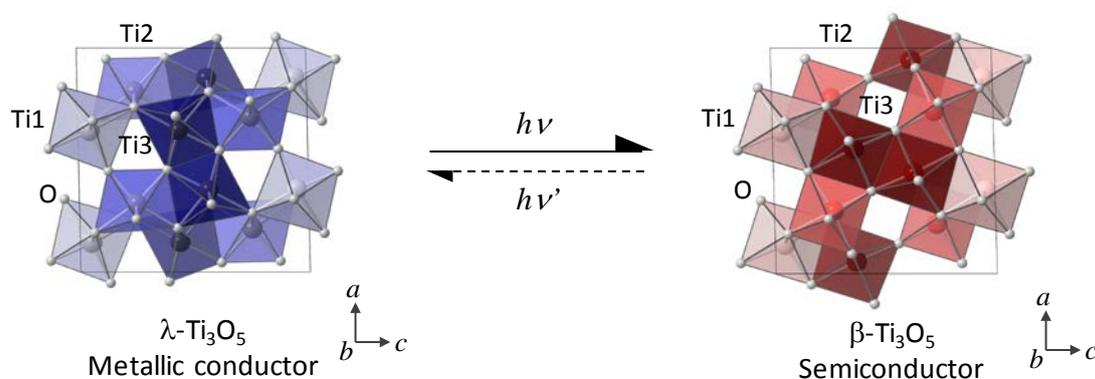
**Figure 1.** Reversible photo-induced metal-to-semiconductor phase transition of  $\lambda$ - $\text{Ti}_3\text{O}_5$  and  $\beta$ - $\text{Ti}_3\text{O}_5$ .
