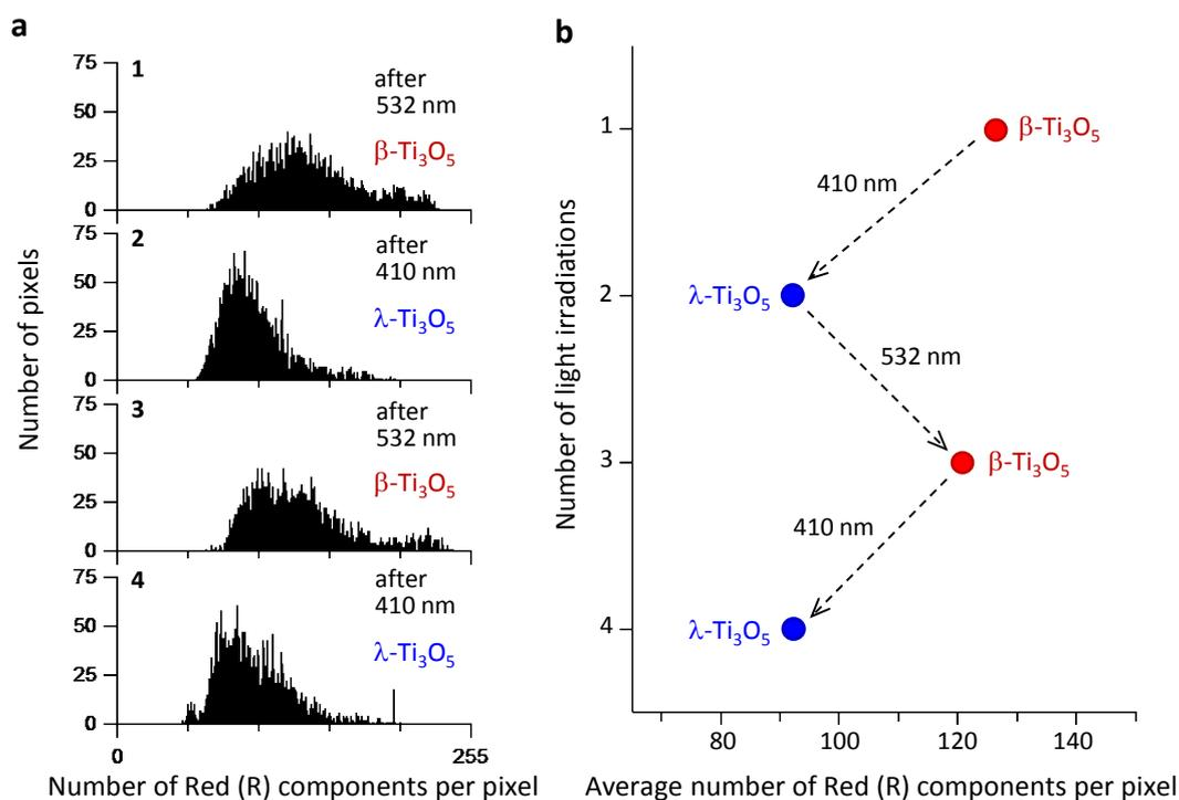
**Figure 3.** (a) Relationship between the number of Red (R) components per pixel and the number of pixels containing the corresponding number of R components in images after 532 nm and 410 nm laser-light irradiation. (b) Plot of the average number of R components per pixel.
