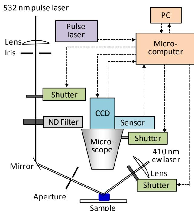
**Figure 2.** Schematic illustration of the experimental setup to evaluate the durability of reversible photo-induced phase transitions.
