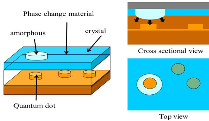
Fig. 1. Principle of local strain application to a QD using a phase change thin film deposited on a QD sample.
