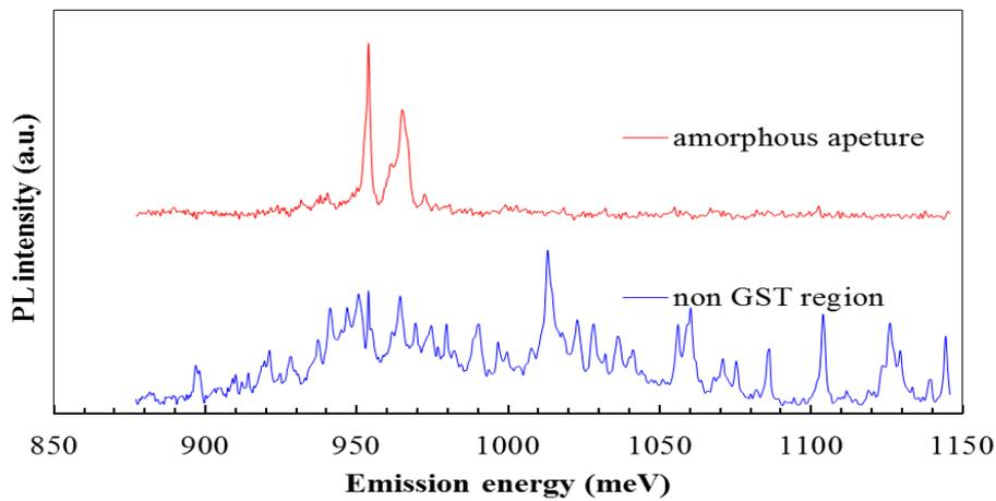
Fig. 3. PL spectra of InAs QDs obtained at non-masked region (blue) and through the amorphous aperture (red).
