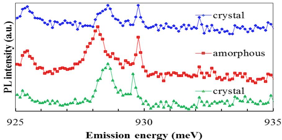
Fig. 4. PL spectra of InAs QDs measured before (green) and after (red) amorphization. The PL peak energy recovered to the original position after recrystallization by laser annealing (blue).
