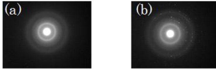
Figure 3: TEM electron diffraction patterns of two different amorphous states: (a) amorphized by single-femtosecond pulse irradiation and (b) amorphized by multi-femtosecond pulse irradiation.
